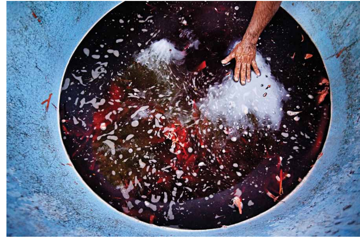
Leather tanning and dyeing process with the bark from a local tree, the Palo Blanco.
